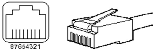
Figure B-6. RJ-45 Cable Connectors: Receptacle and Plug
