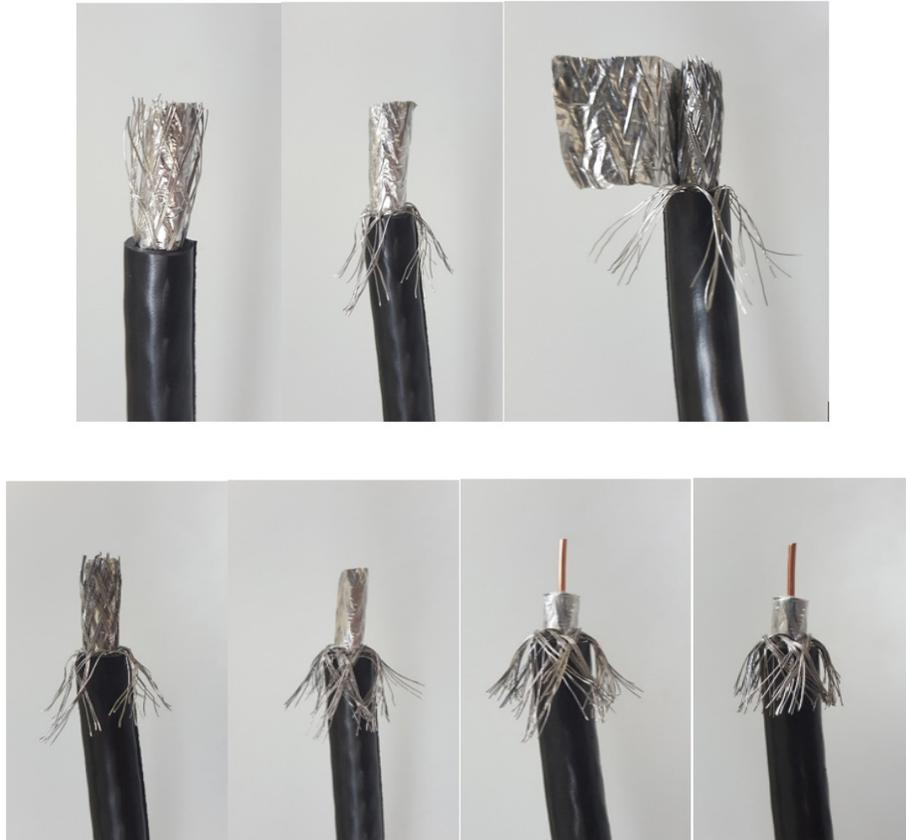
**Figure B-3. Procedure to Cut the Quad Shield Cable**
