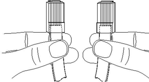
Figure B-7. Holding the RJ-45 Cable Connectors
