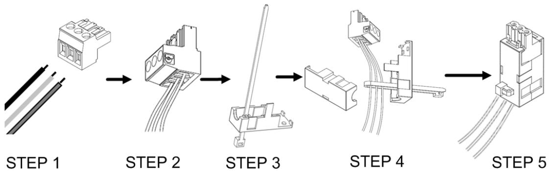
**Figure C-1. DC-DC Power Supply Assembly at a Glance**
