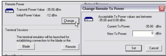
Figure 47. iMonitor Change Remote Tx Power Dialog Box
