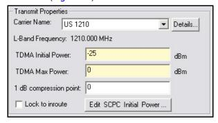
Figure 49. iBuilder Remote Information Tab: Setting TDMA Initial and Max Power
