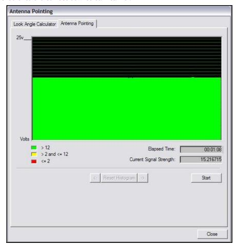
Figure 36. Locking on to a Carrier Stream
