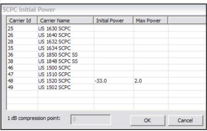
Figure 51. SCPC Initial Power Dialog Box: Setting SCPC Initial and Max Power
