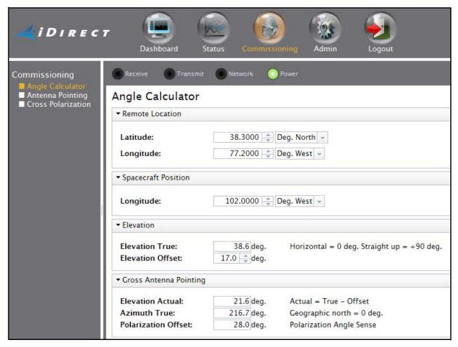
Figure 38. Evolution X1 Angle Calculator
