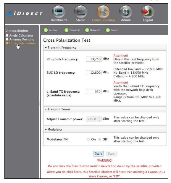
Figure 42. Evolution X1 Cross Polarization Web Page
