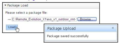
Figure 28. Loading an Evolution X1 Image File
