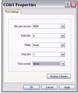
Figure 3. HyperTerminal COM1 Properties Dialog Box
