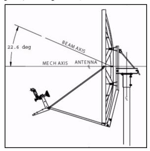
Figure 32. Antenna Elevation Offset
