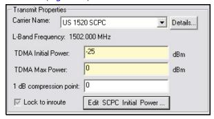
Figure 50. iBuilder Remote Information Tab: Transmit Properties
